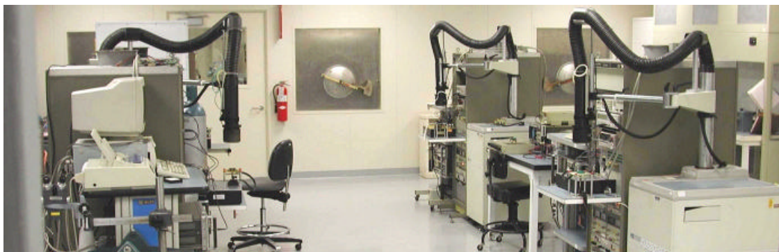
Class 10,000 clean room- Electrical Inspection Area
